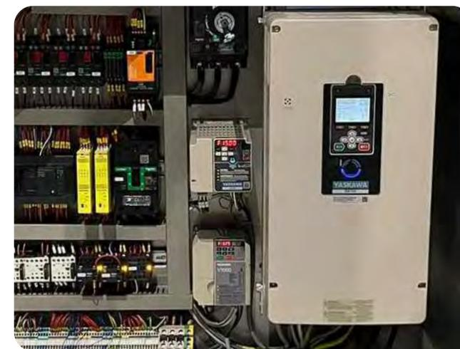
**Soft start and stop of knives, bowl and extracting disc** (optional) by mean of speed drives.
