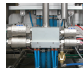
DOUBLE VALVE VACUUM & GAS SYSTEM
