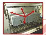
**Four-Sided Moving Wash Frame** — Completely surrounds the items being washed with multi-directional high pressure spray jets which blast away dirt and grime from all four sides. The Jeros Wash Frame provides complete corner to corner coverage eliminating "dead corners" as it repeatedly travels from back to front and front to back inside the wash chamber.
