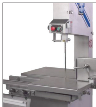
Picture illustrates Sliding Table with Multidirectional Setting Adjustment and Start/Stop Controls on Visible Eye Level
