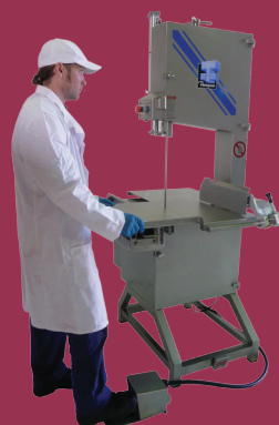
Foot Control depressed Bandsaw Blade Guard raises to Pre-selected Height
