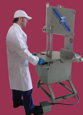
Foot Control Released Bandsaw Blade Guard comes down
