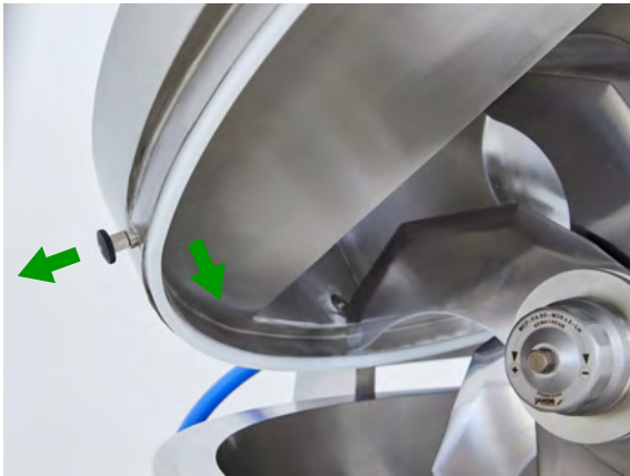
Removeable lid/bowl friction band to facilitate cleaning.
