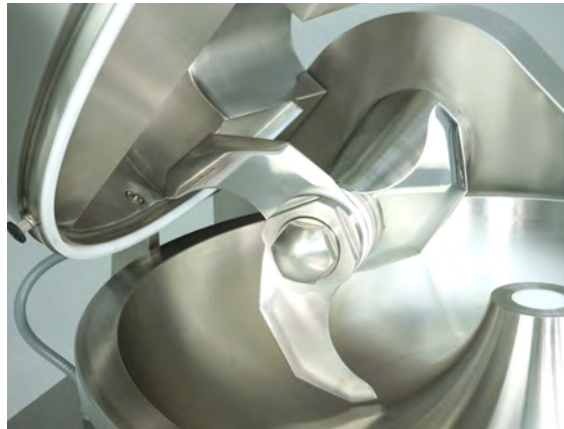
2 compensation rings for use with 3 knives.
