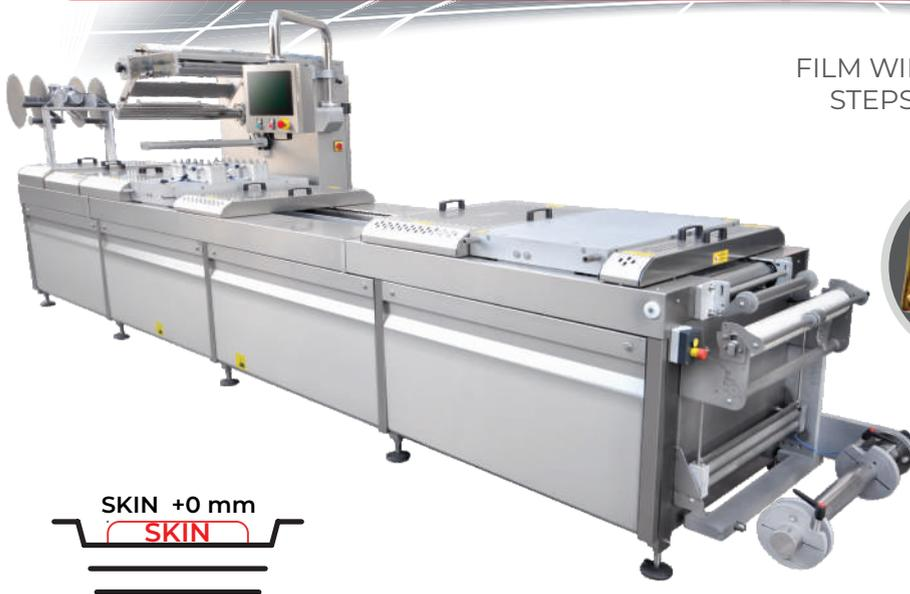
FILM WIDTH FROM 100 TO 670 mm. ANY MEASURE
